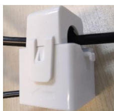
FIG.8 Install the CT
